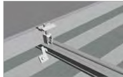
Detail side fixing clip and module clamp
